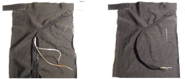
Fig. 3. Vibration motor sewed on elastic fabric.
