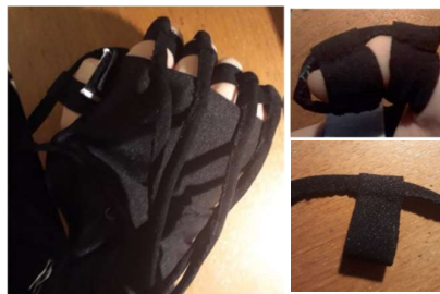
Fig. 4. Elastic "runner" joint stitched around a sensor cable
