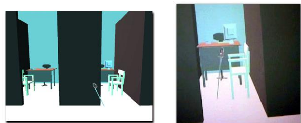
Figure 16 : Cane simulation – Indoors (user wearing the CyberGrasp back-pack)..
