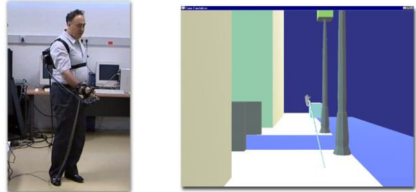
Figure 15 : Cane simulation - Outdoors (user wearing the CyberGrasp back-pack).
